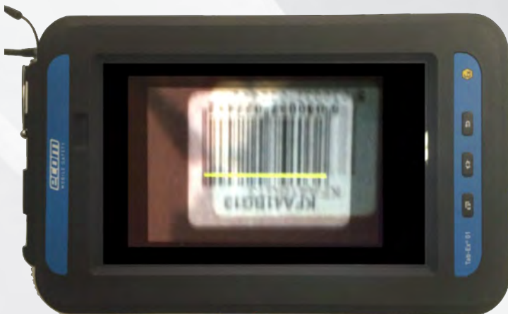
FLANGE TAG BAR/QAR CODE SCANNING
