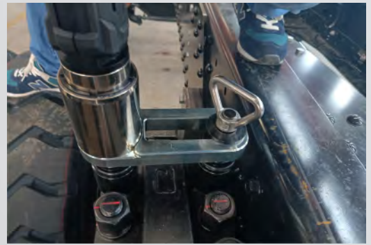
Sliding Reaction Arm
